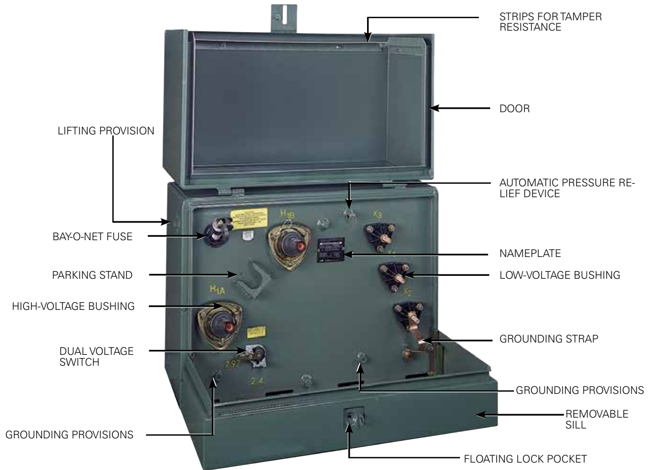
Figure 1. Shrubline single-phase pad-mounted transformer.
