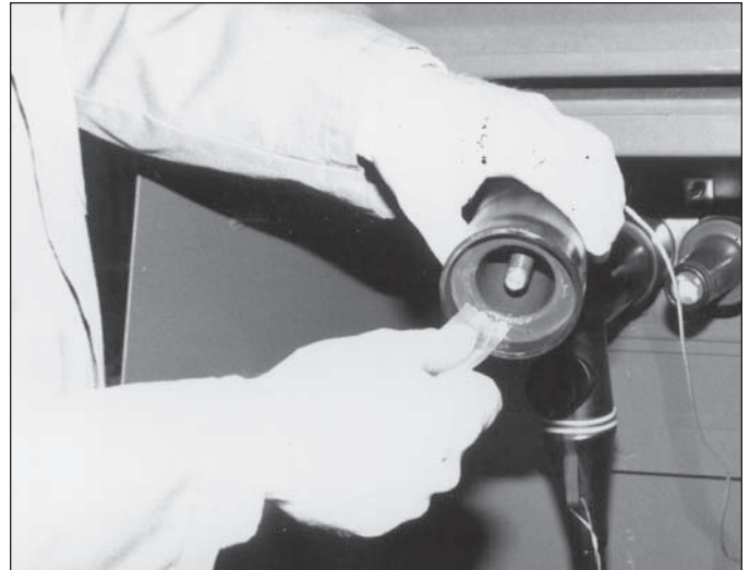
Figure 3. Clean and lubricate cap and bushing mating interfaces.
