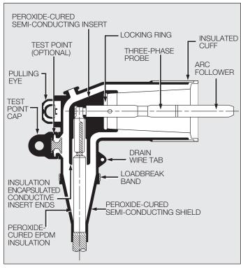
Figure 1. Line illustration of 200 A 35 kV Class Elbow.
