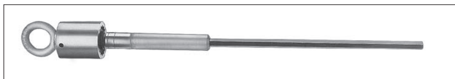
Figure 7. Catalog Number TQHD625 The Torque Tool is required to check the torque of a 15 kV Class T-OP II deadbreak connector or bushing adapter when it is installed on a 600 A bushing interface. It is precision calibrated and hotstick operable.
