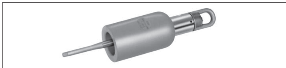
Figure 8. Catalog Number OTTQ615 The combination Operating and Test/Torque Tool is used with a hotstick to test for circuit de-energization and to install and remove a 15 kV Class LRTP equipped connector from an apparatus tap. The standard tool is equipped with a molded EPDM rubber cap and torque limiter to allow proper tool seating and gripping of the T-OP II connector. It also ensures that the connector has been properly torqued into the mating bushing.
