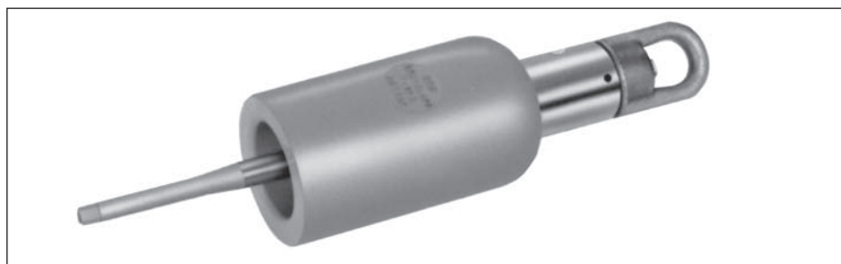
Figure 8. Catalog Number OTTQ625 The combination Operating and Test/Torque Tool is used with a hotstick to test for circuit de-energization and to install and remove a 25 kV Class LRTP equipped connector from an apparatus tap. The standard tool is equipped with a molded EPDM rubber cap and torque limiter to allow proper tool seating and gripping of the T-OP II connector. It also ensures that the connector has been properly torqued into the mating bushing.
