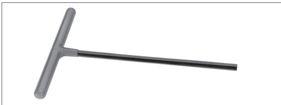
Figure 6. Catalog Number TWRENCH The T-Wrench is used to install the Loadbreak Reducing Tap Plug into the compression connector and T-body.
