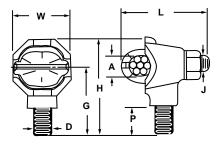
Bodies are cast from high conductivity, high strength copper alloy with cast high strength bronze eyebolts. Steel nuts and lockwashers are standard on all clamps. For silicon bronze hardware, suffix catalog number with "-SBH." Example: GSE-C1-SBH. The HGSE provides a hex or square shoulder for wrench tightening. Its flat surface also acts as a seal to the tank. The GSE may be tightened by using a wrench on the body.
