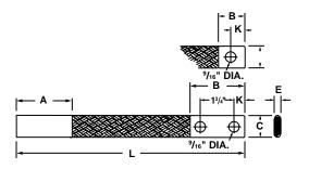
Highly flexible leads suitable for use wherever it is necessary to take up expansion. Made of flat, extra flexible, tinned, pure copper, with tin plated, seamless, pure copper ferrules cold pressed on each end. Inside ends of ferrules are rounded to prevent chafing of strands.
